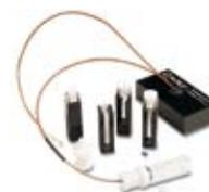
The Temperature Probe accessory measures the temperature inside the cuvette.
